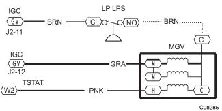
Fig. 30 - LP Supply Line Low Pressure Switch Wiring
